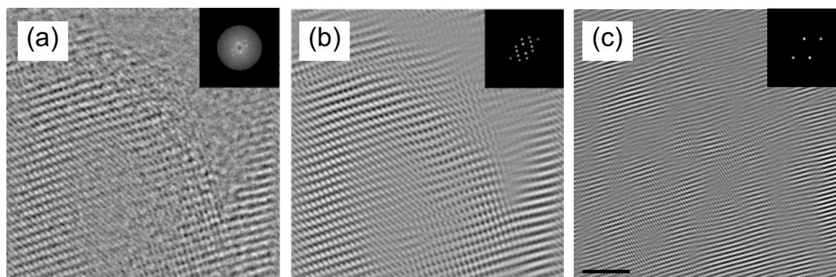
**Figure 2.** Atomic Resolution TEM images of the perovskite degraded for 14 days (a) exit wave reconstruction, (b) FFT (inset) and IFFT of the perovskite and (c) FFT (inset) and IFFT of  $\text{PbI}_2$ .
