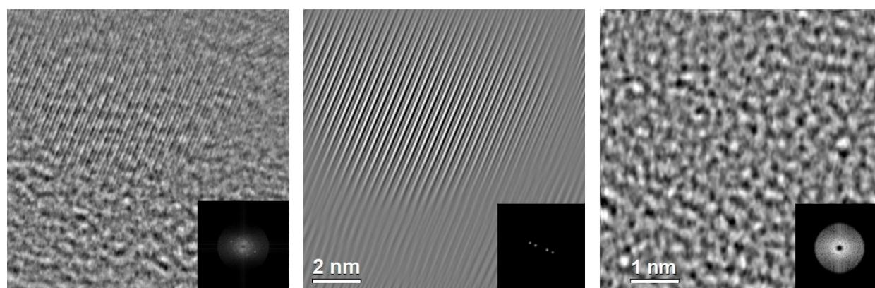
**Figure 3.** Atomic Resolution TEM images of perovskite degraded for 30 days (a) exit wave reconstruction, (b) FFT (inset) and IFFT of the perovskite and (c) FFT (inset) and IFFT of the amorphous region.
