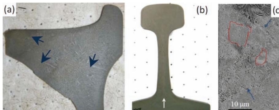
Figure 3—Macro etch of cross sections of a commercial (a) wheel (arrows identifying dendrites), (b) rail (arrow pointing to the partition/segregation line), and (c) crystalline structure from a rail steel showing a fully pearlitic microstructure. The red lines depict the pearlite colony size and the blue arrow point to the prior-austenite grain boundary, which in this case is picked out by pro-eutectoid cementite
