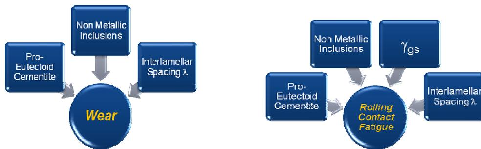
**Figure 7.** Main microstructural factors responsible for the performance of rail steels, where  $\gamma_{gs}$  is the austenite grain size.
