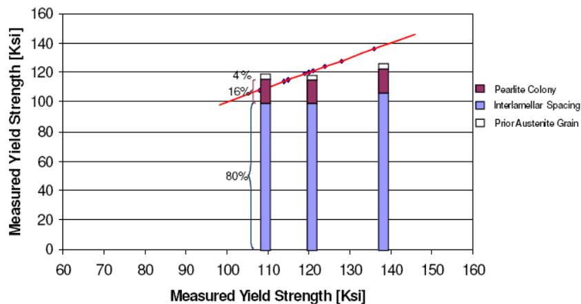
**Figure 5.** The bar height represents the total contributions of microstructural factors to the yield strength of rail steels.
