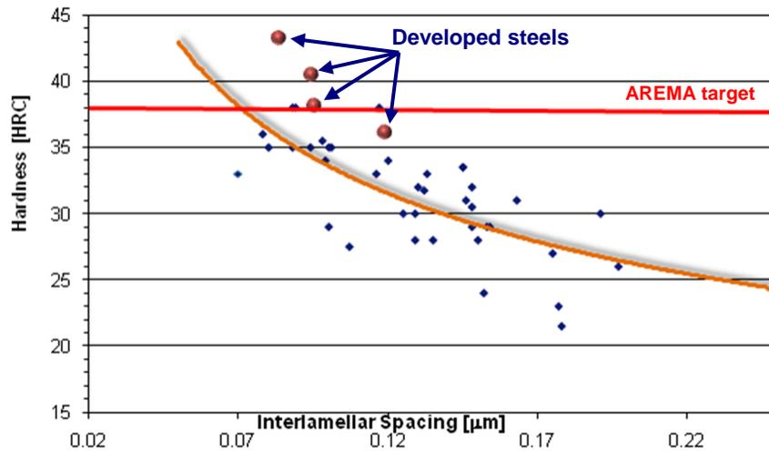
**Figure 10.** Hardness values of premium rail and the developed steels
