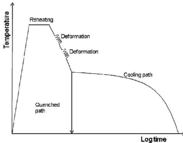
**Figure 2.** Schematic representation of general thermomechanical process.
