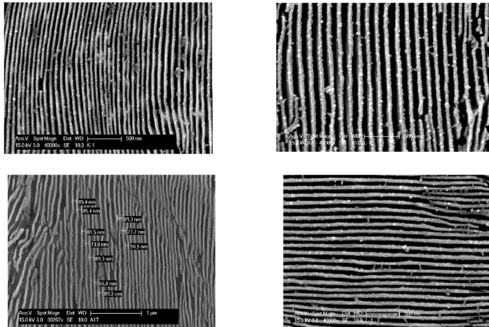
**Figure 3.** Typical lamellae of cementite in a pearlitic microstructure from different premium rail steels.
