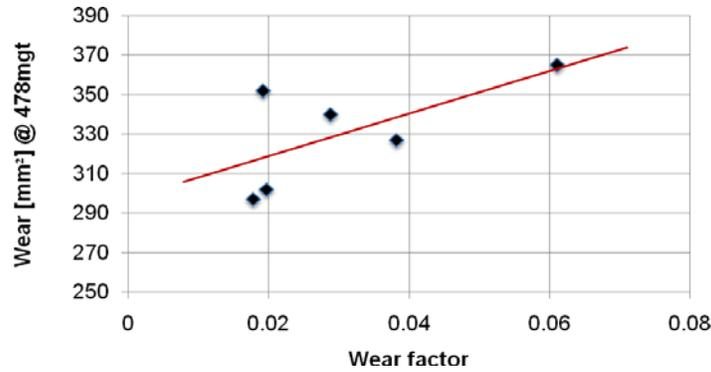
**Figure 8.** Relation between the wear behavior of rail steels and microstructural factors.
