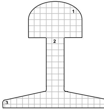
**Figure 1** Rail profile, sample obtained locations.
