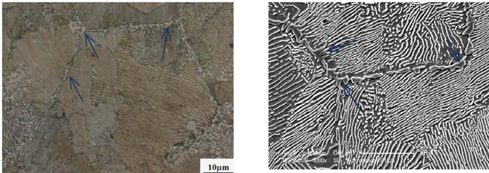
**Figure 6.** Optical and SEM micrograph showing the presence of pro-eutectoid cementite in a rail steel sample.
